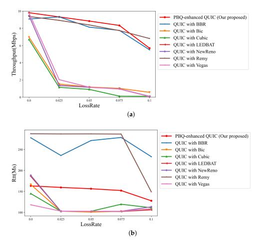
**Figure 9.** Link quality of schemes across different packet loss rates with flow number 2: (**a**) throughput; (**b**) RTT.
